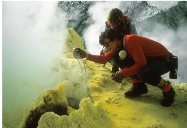
Gas sampling at fumaroles at the summit of Mount Bakers, US state of Washington.
